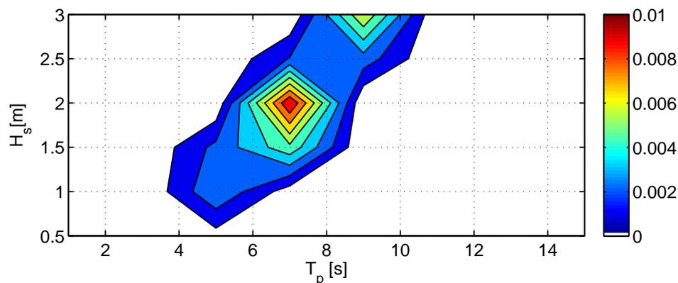
**Fig. 7:** Example contour plot of annual accumulated fatigue damage for mooring. Colour scale denotes accumulated fatigue D damage for one year, taken from [14].
