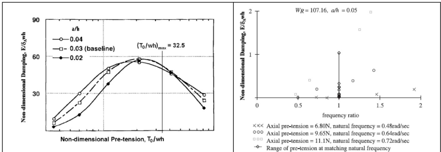
**Fig. 1:** Mooring line damping variation due to changes in pre-tension for different amplitude to water depth ratio.
