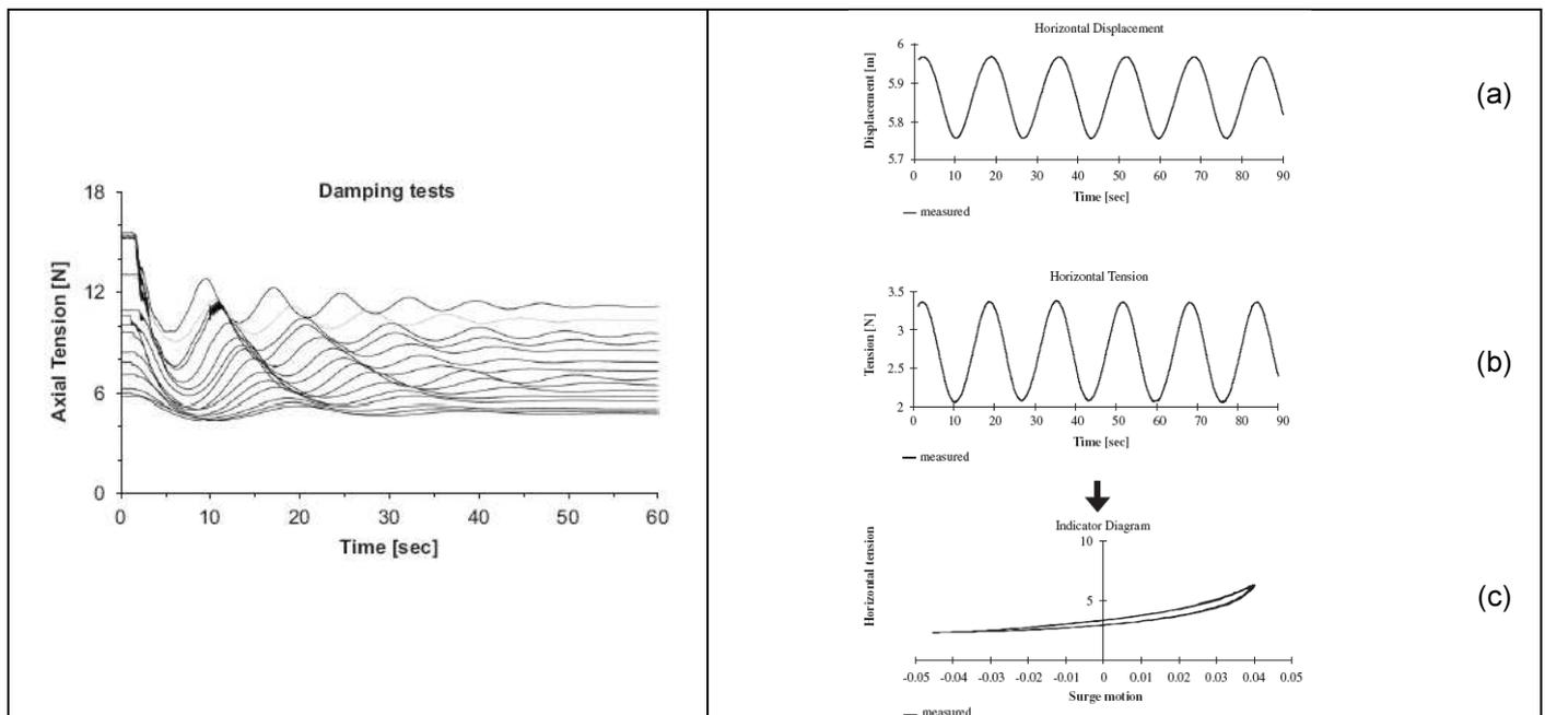
**Fig. 3:** Decaying motion for the same mooring configuration at different pre-tensions [8]
