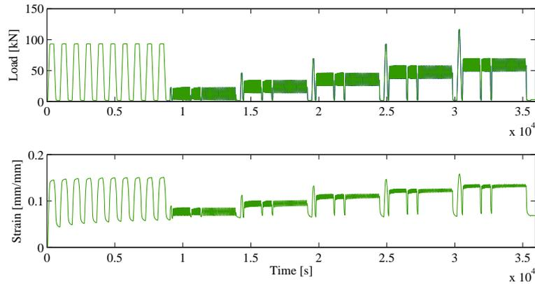
**Fig. 5:** Example applied load and measured strain of a nylon mooring rope sample
