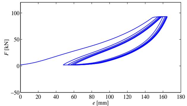
**Fig. 6:** Load-extension loop from rope testing
