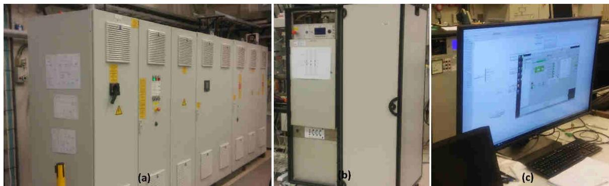
Figure 2.1: Laboratory facilities. (a) Grid emulator, (b) MMC and (c) computer interface
