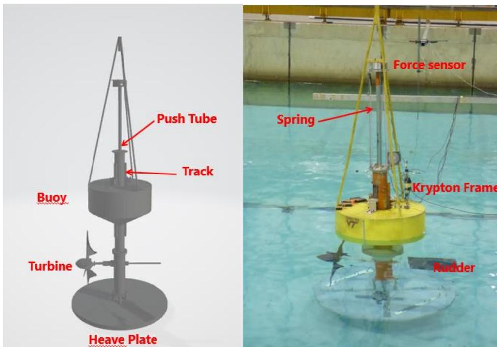
Figure 1: Model of Hybrid wave-current energy converter. 3-D model(left) and hardware for testing(right)
