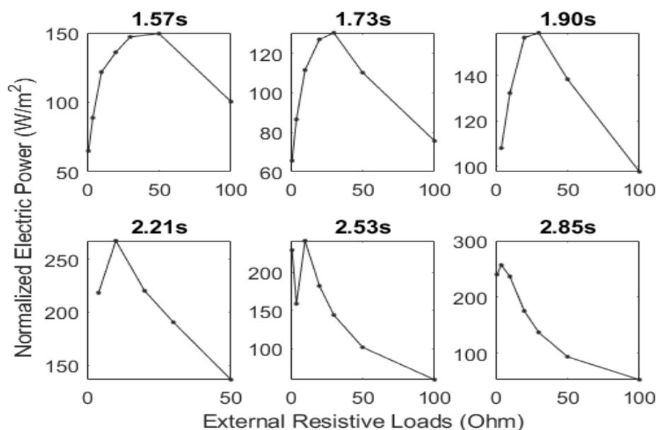
Figure 5: Normalized electric power of point absorber under regular wave excitation
