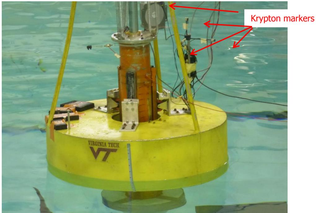
Figure 4: Markers for motion measurements
