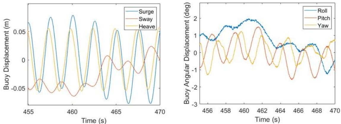
Figure 6: Six degrees of freedom motions of buoy structure. Surge, sway and heave motion (left). Roll, pitch and yaw motion (right).
