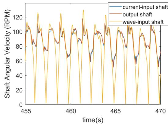
Figure 7: Angular velocity of input/output shafts connecting point absorber, turbine and DC generator.
