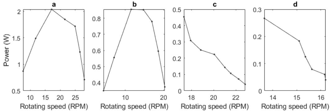
Figure 5: Turbine performance under different conditions. a) 0.6m/s fluid velocity with planetary gearbox between turbine and PTO. b) 0.5m/s fluid velocity with planetary gearbox. c) 0.5m/s fluid velocity without planetary gearbox. d) 0.4m/s fluid velocity with planetary gearbox.
