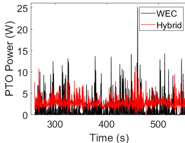
Figure 8: Comparison on output electric power between hybrid converter and WEC
