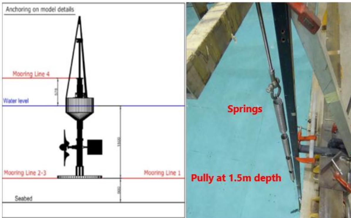
Figure 2 – Implantation of mooring lines (dimensions are given in mm model scale)
