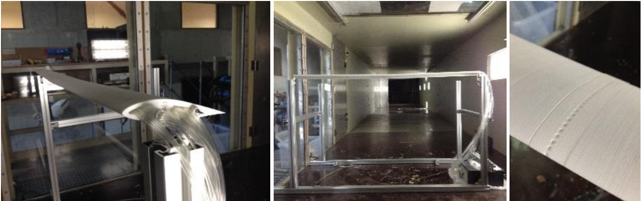
Figure 2.2 – View of the 0.125 chord model aerofoil at the CRIACIV wind engineering Lab.
