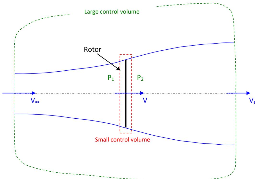
**Figure 2: Unconfined one-dimensional flow through a horizontal-axis turbine**
